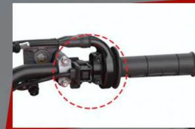
HRC Launch Control
