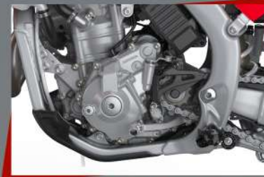
249 cc Liquid-cooled, 4-Stroke Single Cylinder DOHC, 5-Speed Manual
