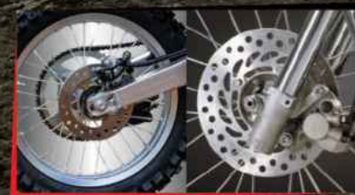
SINGLE FRONT AND REAR DISC BRAKE
