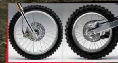
19-INCH FRONT AND 16-INCH REAR WHEELS
