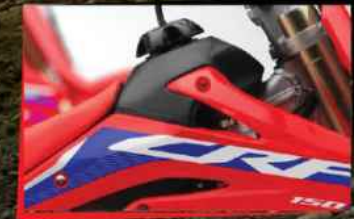
4.3 LITERS FUEL TANK CAPACITY
