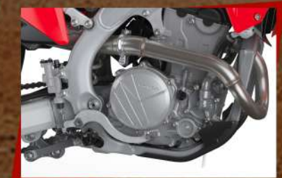
450cc Liquid-cooled, 4-Stroke Single Cylinder SOHC, 5-Speed Manual
