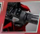
HAZARD & ISS SWITCH
