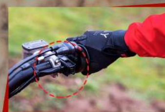
HRC Launch Control
