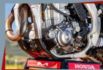
450cc Liquid-cooled, 4-Stroke Single Cylinder Uni-cam 5-Speed Manual
