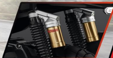
Subtank Rear Suspension
