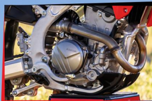
LIQUID-COOLED, 4-STROKE SINGLE CYLINDER, DOHC
