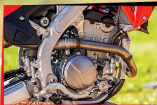
LIQUID-COOLED, 4-STROKE SINGLE CYLINDER, DOHC
