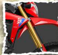
LONG TRAVEL INVERTED FRONT FORK (SHOWA BRAND)
